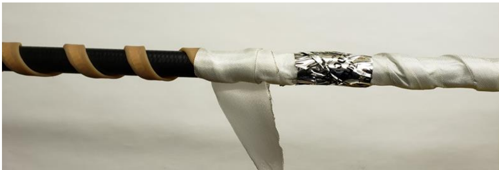
FIGURE 3 - Hose wrapped with Briskheat heating tape and fiberglass cloth tape
