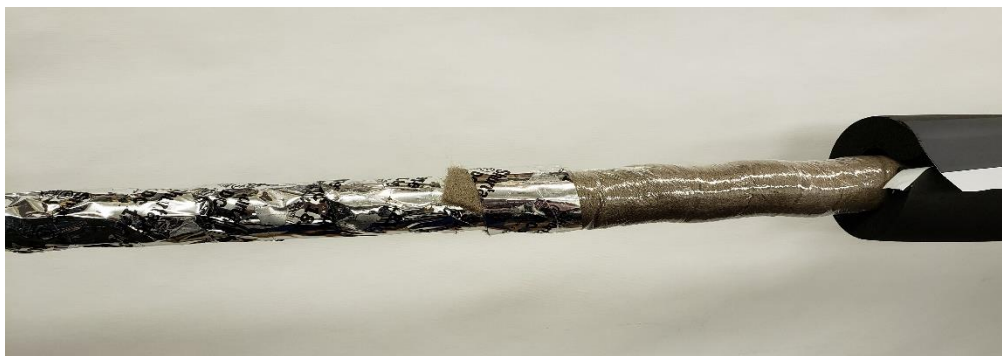
FIGURE 4 - Hose wrapped with foil tape
