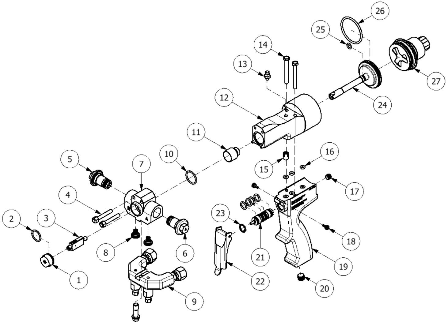
**NOTE:** WHEN ASSEMBLING BE SURE TO APPLY GREASE TO **ALL** O-RINGS. THIS ENSURES GOOD PERFORMANCE AND REDUCES RISK OF GUN MALFUNCTION.
