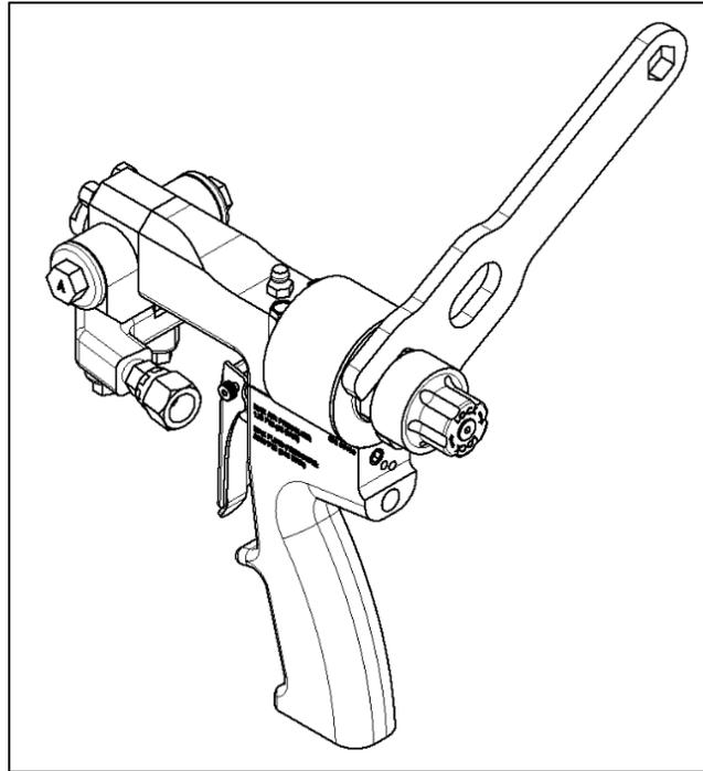
8. Using the Nut Driver provided, remove the gun block mounting screws and disconnect the Gun Block.
