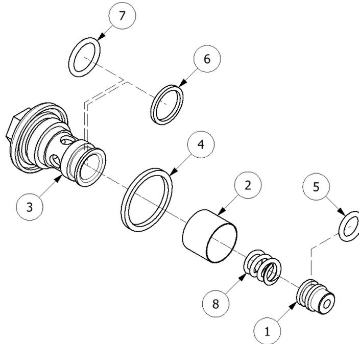
**NOTE:** WHEN ASSEMBLING BE SURE TO APPLY GREASE TO **ALL** O-RINGS. THIS ENSURES GOOD PERFORMANCE AND REDUCES RISK OF GUN MALFUNCTION.
