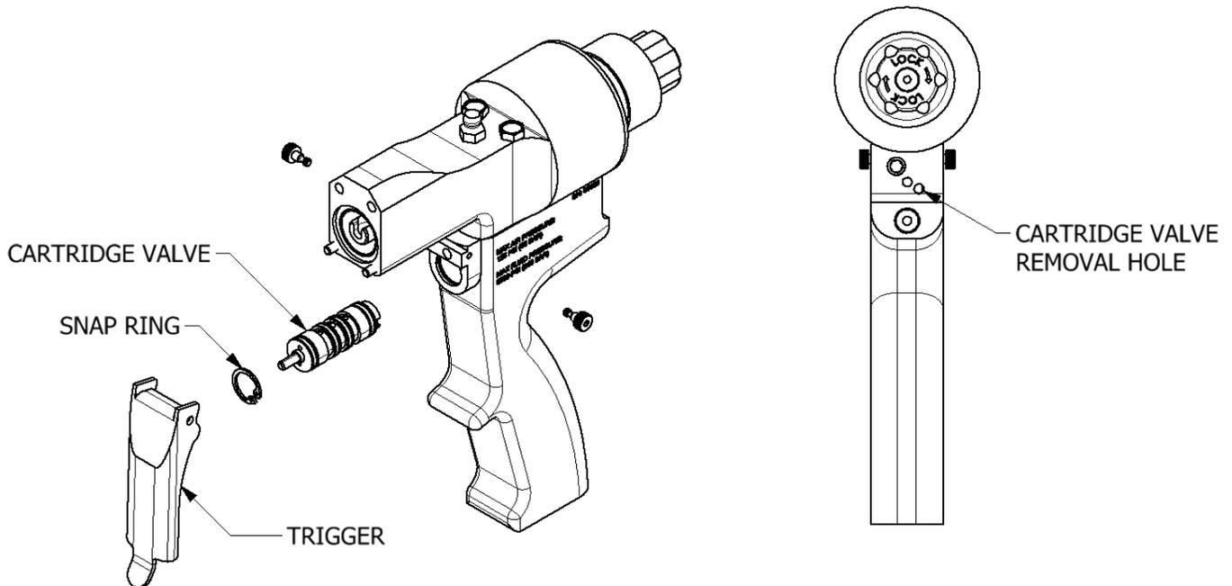
1. Remove the trigger from the handle.
