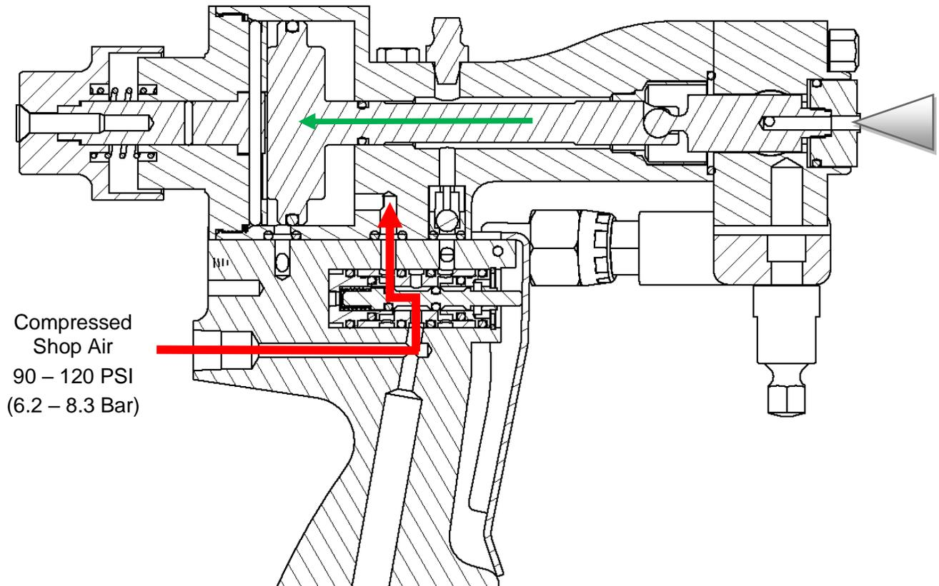
1. Compressed **dry air** is directed through the cartridge valve and into the front, filling the cavity and pushing the Piston and Chamber backwards.
