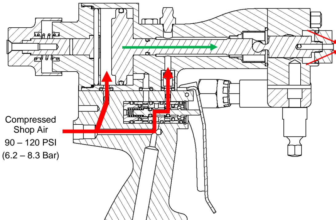
2. The air is directed through the cartridge valve and into the Rear of the Piston in the Air Cylinder, moving the Piston (and Mixing Chamber) forward to the **CLOSED** position.
