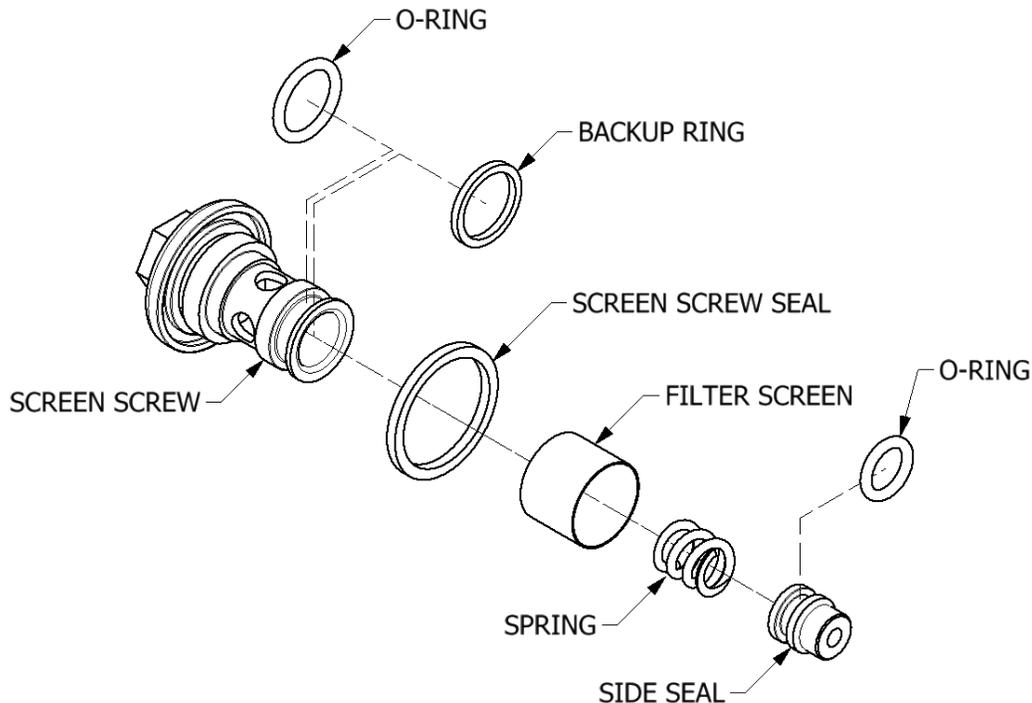
**CAUTION!** To avoid possible contamination by the residual chemical inside the Gun do not interchange the Isocyanate (A) parts with the Polyol (R) parts. The Isocyanate (A) side is identified with an (A) on the Screen Screw Head and the Polyol (R) side is marked with an (R) on the Screen Screw Head. The Gun Block is also marked with (A) and (R) designation.
