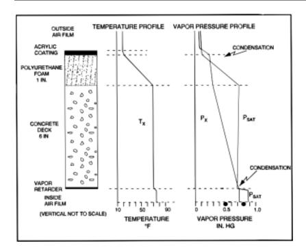
The table in Step 5 summarizes all the information and calculations from Steps 1-4. In addition, the last column,  $P_{sat}$ , gives the saturated vapor pressure for the temperature at the corresponding surface. The saturated vapor pressure is read off Table 2 for the appropriate surface temperature  $(T_x)$ .
