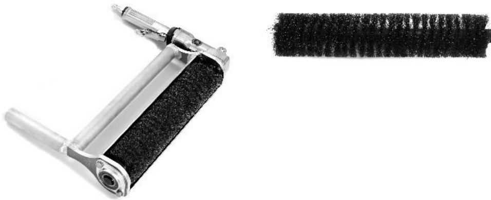
Figure 20 - Scarifier with wire-wheel brush (air driven)
