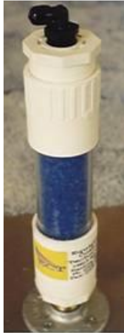
Figure 4 - Silica Gel Dryer mounted in 3/4" hole of A-side Drum
