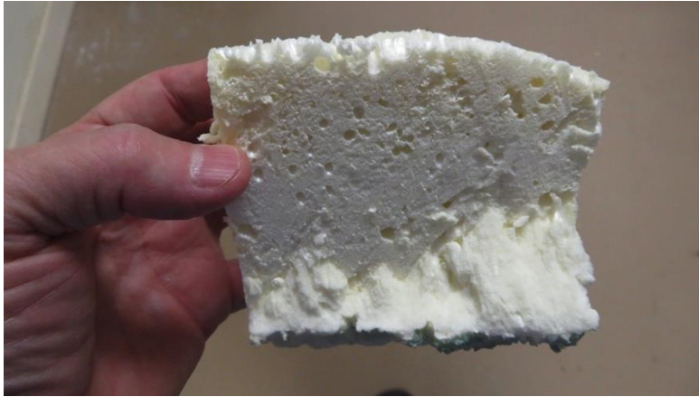
Figure G6-4: Darker color & soft foam in the center, blowholes and strong odor indicates excessive exothermic heat.
