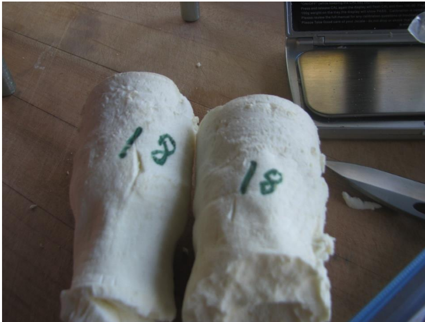
Figure G6-3: If the samples contract overnight, then the lifts were too thick.
