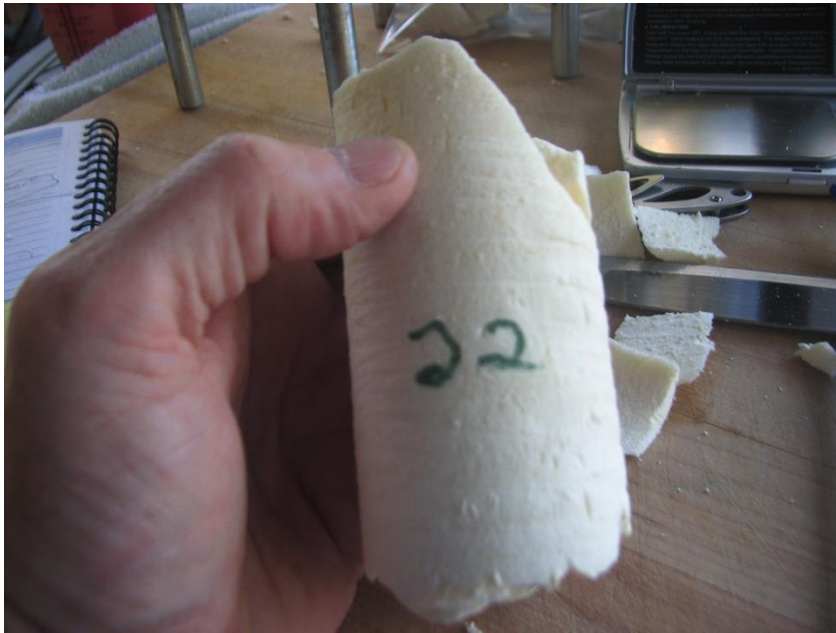
Figure G6-2: Core samples of the foam can verify quality foam. Check for good cell structure, compressive strength and dimensional stability.
