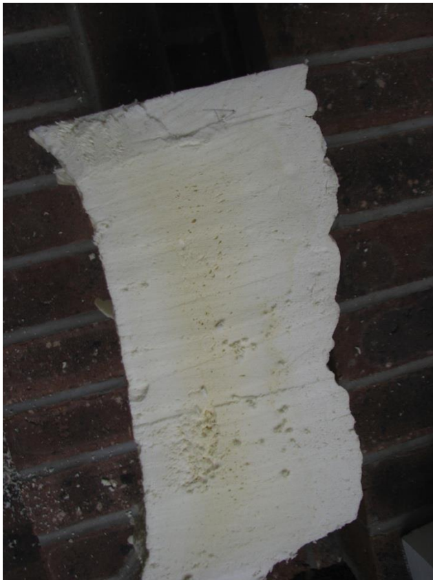
Figure G6-3: If the samples contract overnight, then the lifts were too thick.
